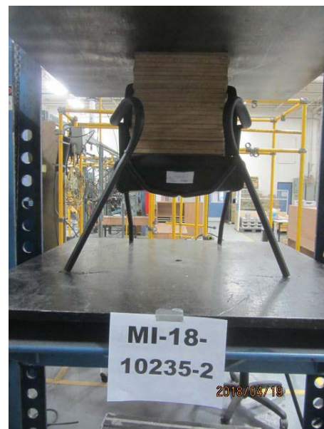
Photograph #3 Chair after peak load reached
